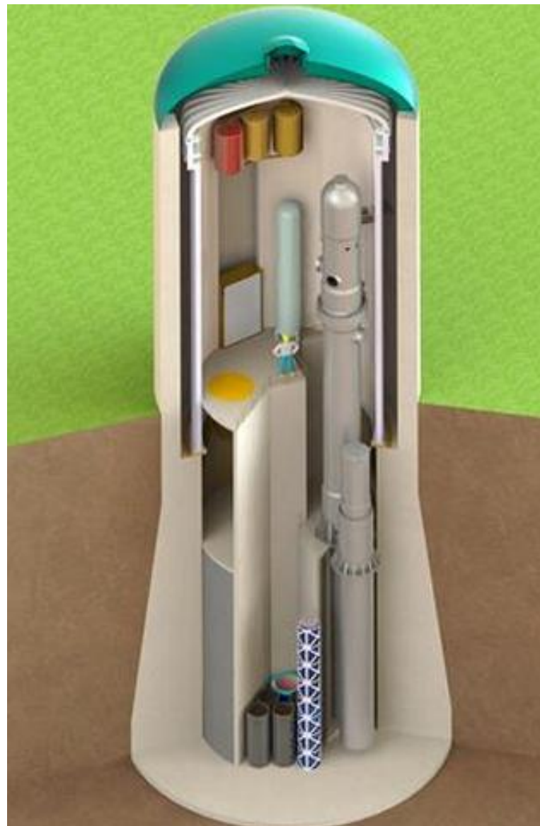
Containment structure and containment enclosure structure
